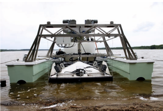
The watercraft unit with its conspicuous underwater module suspended in the surface watercraft dock.
